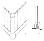
Figure 1 A drawing of stave construction done by Hörður Ágústsson architect. (Ágústsson, H., 2004, bls. 128)
