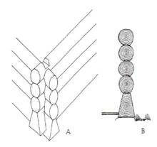
Figure 2 A drawing of a stokkverk by Hörður Ágústsson architect. (Ágústsson, H., 2004, p. 128)
